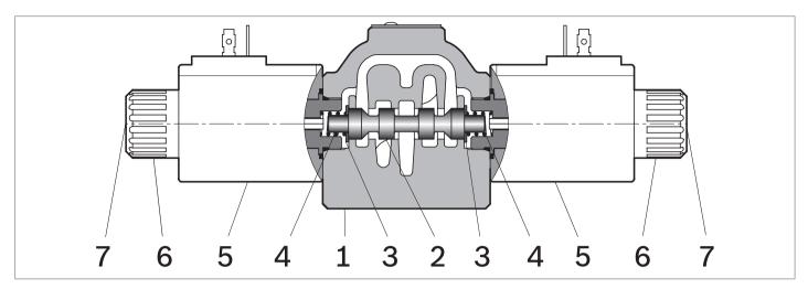
The directional valves LC1F\_DZ are compact direct operated solenoid valves which control the start, the stop, the direction of the oil flow. They basically consist of a housing (1) with a control spool (2), one or two solenoids (5), and one or two return springs (4).
