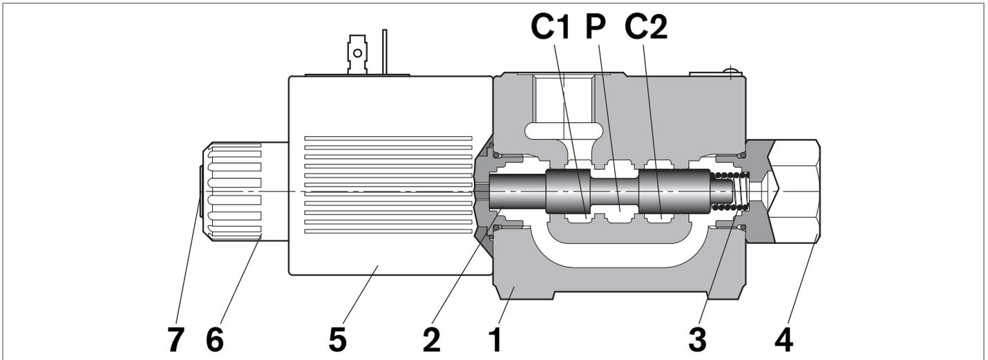
A valve basically consists of a housing (1), a control spool (2), a return spring (3) and a solenoid (5). It is designed to select which one of two circuits (C1 or C2) is to be supplied with the oil delivered from one single hose (P): with spool in position "0", when the solenoid is de-energized, the flow goes from P to C1, with spool in position "1", when the solenoid is energized the flow goes from P to C2.
