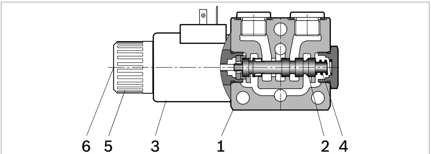
The sandwich plate design valve elements L808103P... are compact direct operated proportional solenoid valves which divert totally or partially the inlet P flow to Tank. These elements basically consist of a stackable housing (1) with a control spool (2), one solenoid (3), and one return spring (4).
