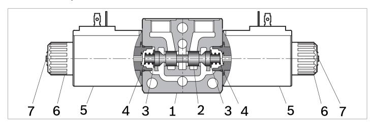
The sandwich plate design directional valve elements L8\_11... are compact direct operated solenoid valves which control the start, the stop and the direction of the oil flow. These elements basically consist of a stackable housing (1) with a control spool (2), one or two solenoids (5), and one or two return springs (4).
