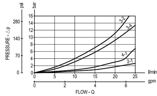
**Version 10 - Direction of flow 3-2** **Version 10 - Direction of flow 3-4**
