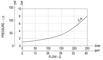
Measured with hydraulic fluid ISO-VG46 at  $36^{\circ} \pm 2 {\circ}C$  (97°  $\pm 36 {\circ}F$ ); ambient temperature 23 °C (73 °F).
