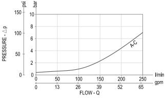
Δp = f (Q) Pressure drop - Flow rate characteristic Lowering (C->A), main stage (3) completely open.
