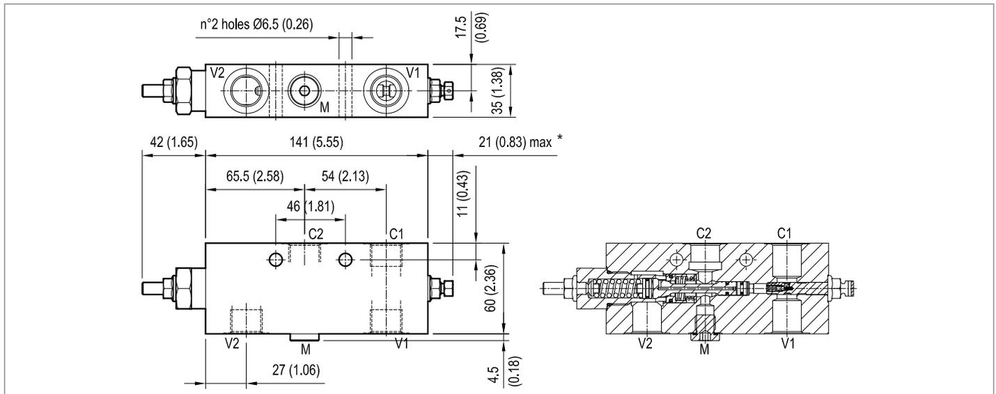
\* The adjusting screw can be completely unscrewed. Do not exceed the indicated protrusion range of the adjusted screw.
