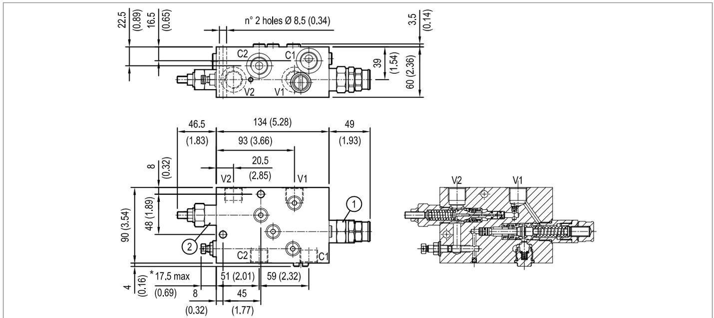
\* The adjusting screw can be completely unscrewed. Do not exceed the indicated protrusion range of the adjusted screw.
