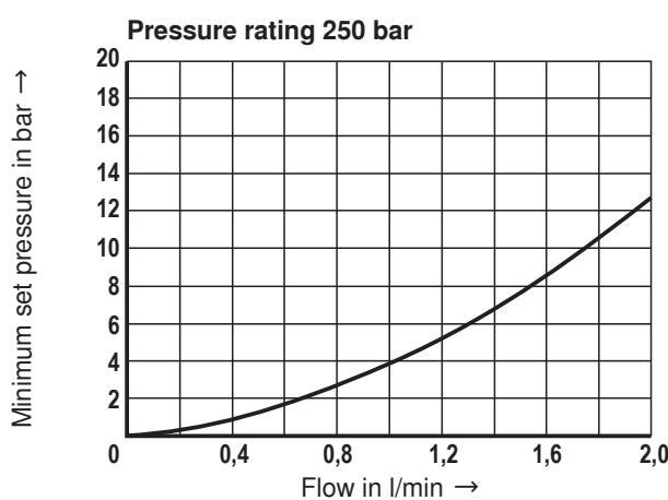
**Characteristic curves** (measured with HLP46,  $\vartheta_{\text{oil}} = 40 \text{ }^{\circ}\text{C} \pm 5 \text{ }^{\circ}\text{C}$  and 24 V coil)
