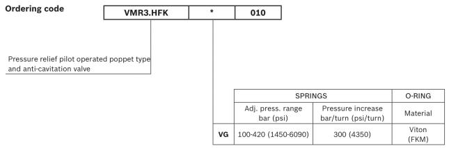
\* Valves are delivered set at pressure setting <25 bar and with adjustment device not tighten. Fine setting to be done by customer. For case of request of factory set valve, please consult factory.
