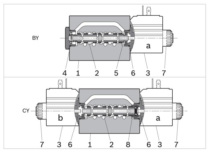
A valve basically consists of a housing (1), a control spool (2), one or two solenoid (3), and a return spring (4).
