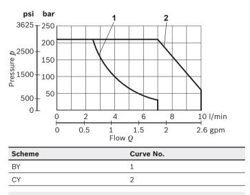
The performance curves are measured with flow going across and caming back.
