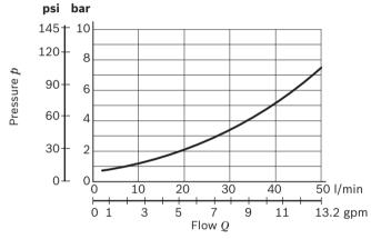
Measured with hydraulic fluid ISO-VG32 at 45° ±5 °C (113° ±9 °F); ambient temperature 20 °C (68 °F).
