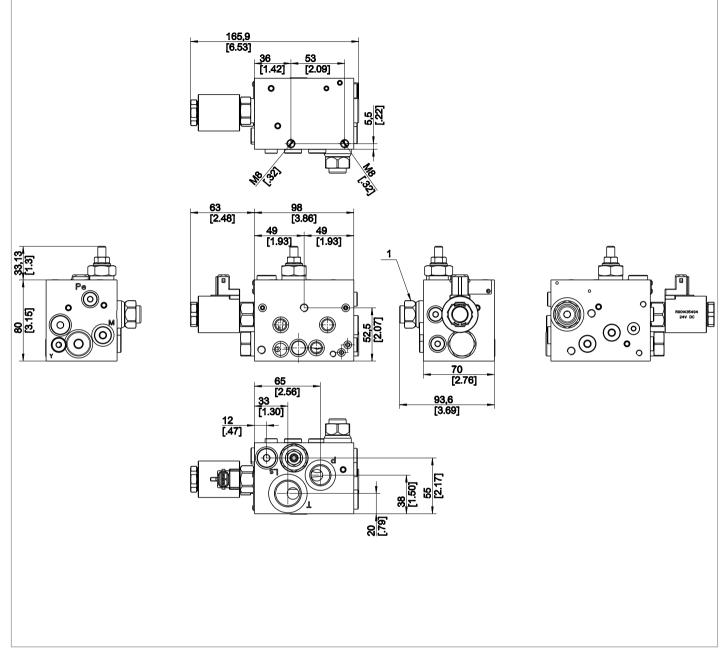
**1** Pressure reducing and relieving valve MHDRDB, optional configuration (refer to RE 18318-55).
