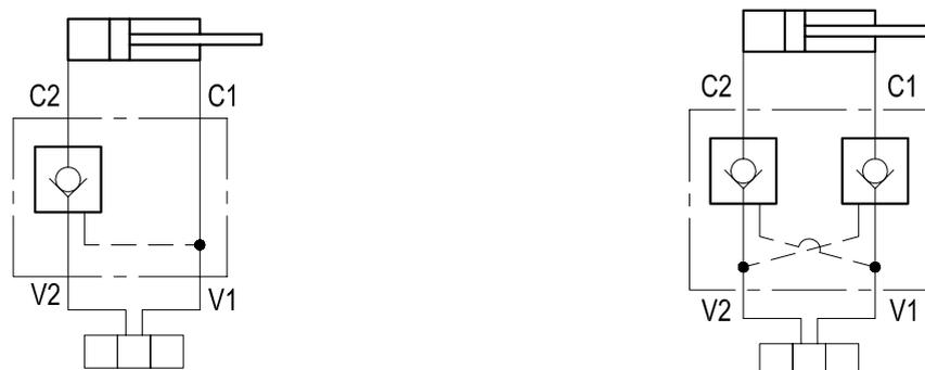
Pilot operated check valve modules are available in SINGLE ACTING and DOUBLE ACTING version: in both cases, one of their basic parameters is the
