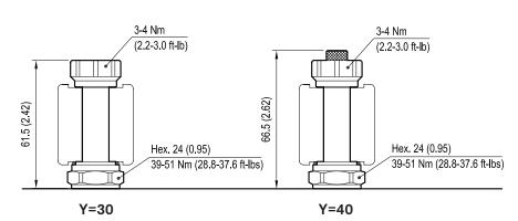
CARTRIDGE TECHNICAL DATA Common cavity: CA-08A-4N Filtration: 25 μm nominal or better
