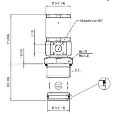
▼ Version 31: Directional control valves hydraulic operated poppet 2-way double lock normally closed - Special cavi-
