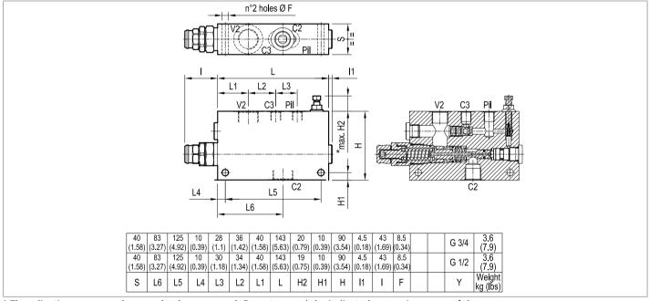
\* The adjusting screw can be completely unscrewed. Do not exceed the indicated protrusion range of the adjusted screw.
