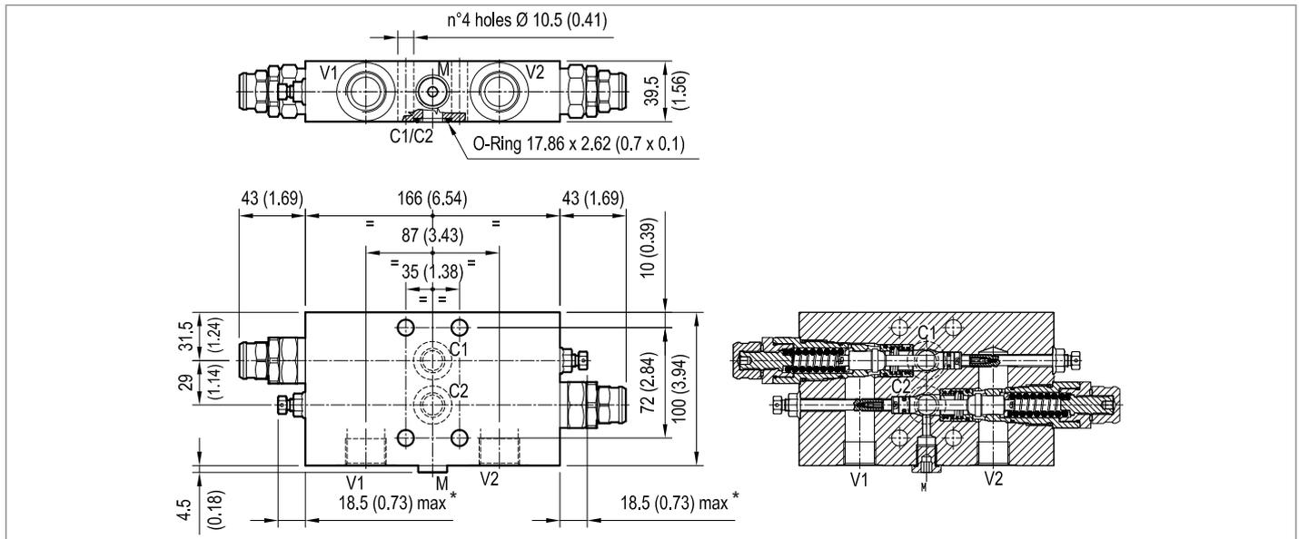
\* The adjusting screw can be completely unscrewed. Do not exceed the indicated protrusion range of the adjusted screw.
