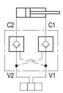
Pilot operated check valve modules are available in SINGLE ACTING and DOUBLE ACTING version: in both cases, one of their basic parameters is the
