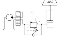
2) In case of load pulling the cylinder rod and valve fitted to the annular chamber
