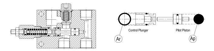
With this counterbalance valve design, the back-pressure Pv at port V2 is additive with the ratio 1 : 1 to the relief setting Pt and with the ratio (R + 1) / R to the theoretical pilot pressure Ppil for piloted opening.
