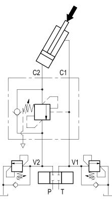
This type of "fully balanced" valves is necessary in a few typical applications and exactly:
