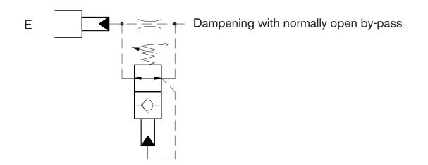
In case of quick lowering, the VEM locks almost immediately and the pressure increase in the pilot chamber is controlled by the dampening screw.
