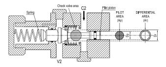
Very compact design providing excellent flow control, good tolerance to oil contamination; internal components developed especially for parts in body (most frequently steel body), but occasionally available also as complete "screw-in cartridges", with various flow capacities ranging from 40 l/min up to 350 l/min.
