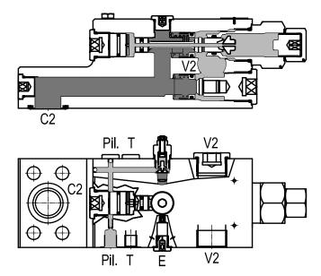
B) Boom holding: the Main Control Valve is in neutral position and no flow is delivered to the cylinder. The pressure induced by the load inside the cylinder pushes back the annular check valves against the seats: the oil the cylinder is locked in a "leak free" mode and the boom is held stationary.
