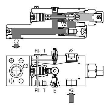
A) *Boom lifting*: the oil delivered by the Main Control Valve reaches port V2, opens the check valves, enters and extends the cylinder through port C2.
