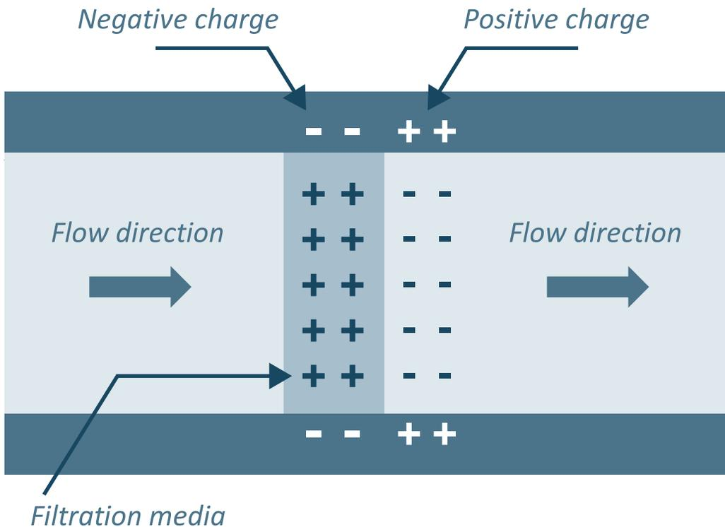
Use of an electrically conductive filter reduces the risk of electrostatic buildup and subsequent discharge, which can damage the filter and allow particles to pass through.
