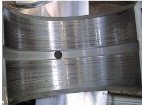
Contaminated hydraulic fluid can lead to damage such as scratches on bearing components and erosion of surfaces due to particles streaming against parts.
